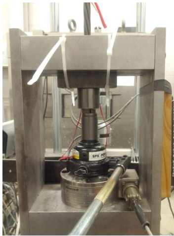
Figure 4.11: Hydraulic Jack Arrangement
