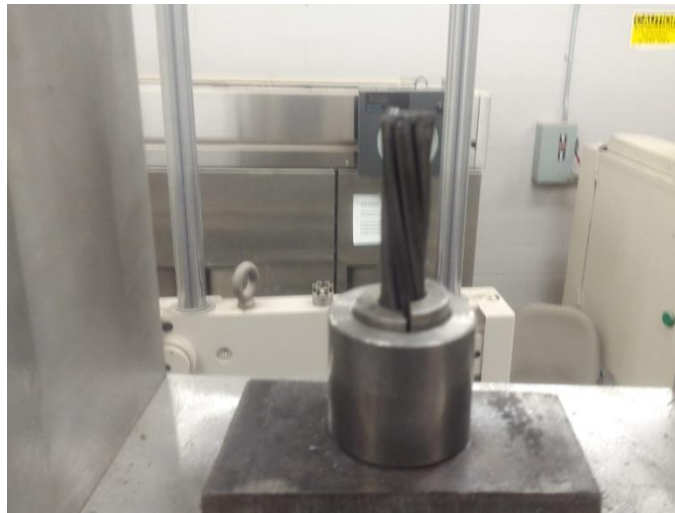
Figure 4.10: Extra Strand Extended Past Anchor
