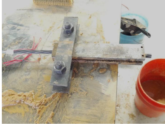
Figure 4.6: Bolted Custom Grips
